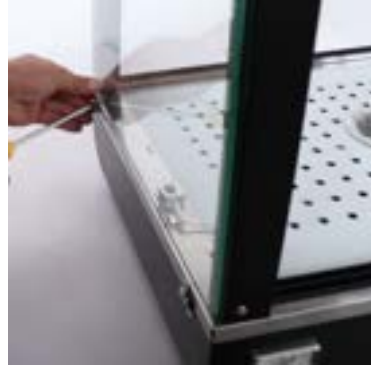
Insert left and right windows and secure them with screws
