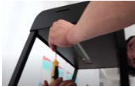
Screw in the top to the base and frame supports
