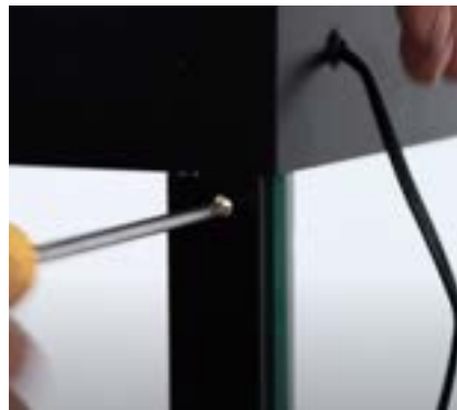
Pull the power plug through the opening at the top then secure in place
