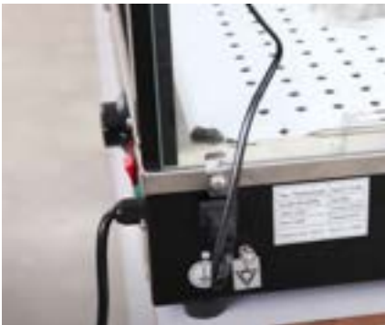
Pull the power plug through the opening at the top then secure in place
