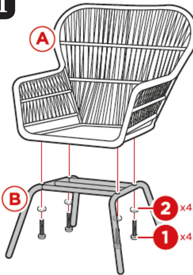
Place the seat on top of the base and secure it with 4 screws and 4 washers. Make sure the screws are tightened.
