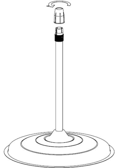
3. Slide the height adapter into the upper standing pole. Then put the upper standing pole into lower standing pole and fasten the height adapter for your desired height of fan.
