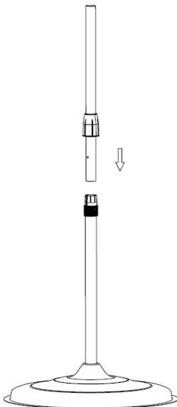
4. Connect the fan head with upper standing pole. Then tighten firmly two sets of screws, washers and nuts at the holes of fan head.
