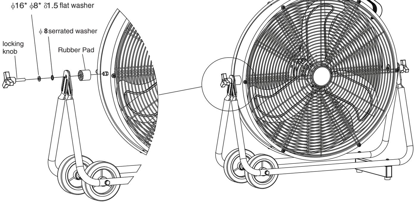
Assemble the base bracket with two side of drum body by fastening the locking knobs, flat washers, serrated washers and rubber pads.
