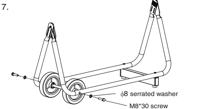
Fastening the wheel assembly into the base bracket by M8\*30 screws and  $\phi 8$  serrated washers.
