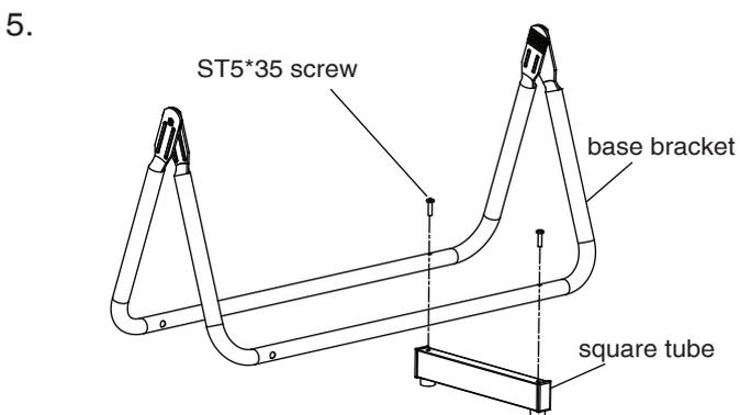
Install the square tube with base bracket by screws ST5\*35.
