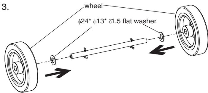
Insert the flat washer and wheel to the wheel shaft
