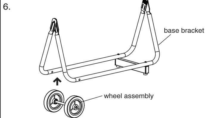
Install the wheel assembly into the base bracket
