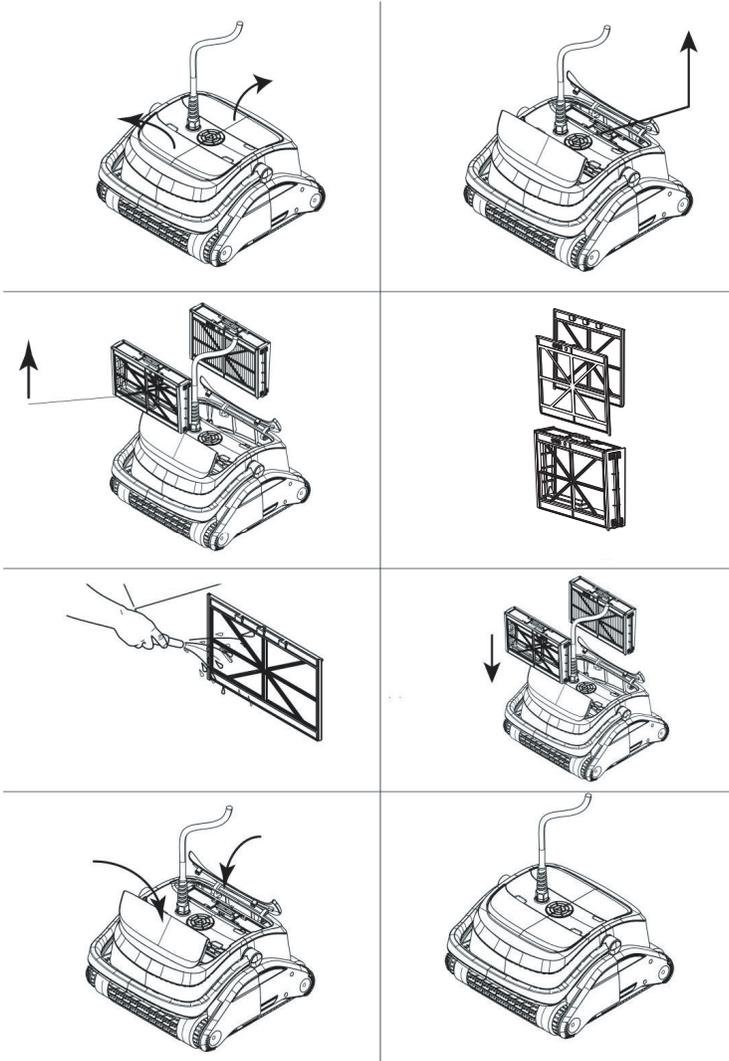
Make sure the power supply is switched off and unplugged.It is highly recommended to clean the filter basket after each cleaning cycle.
