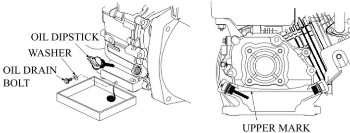
4. Reinstall the oil dipstick and tighten it.
