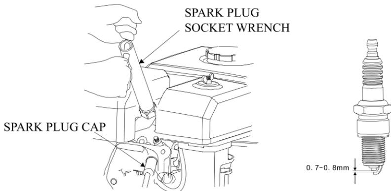
4. Check if the spark plug gasket is in good condition. In order to avoid damage to the thread in the cylinder head, screw in the spark plug carefully by hand.
