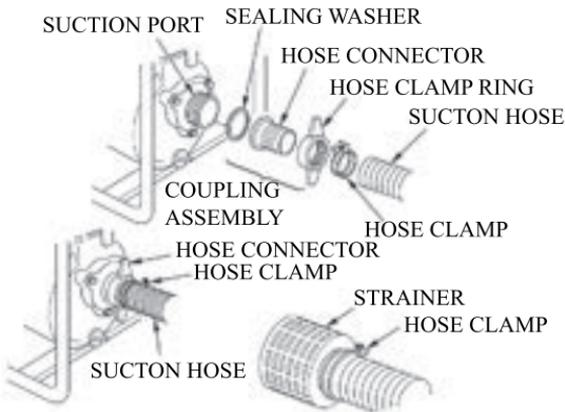
Hose dimension should be longer than water suction port dimension.
