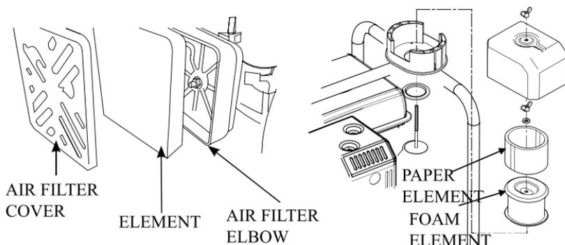
Screw off butterfly nut and remove air filter housing, If the element is
