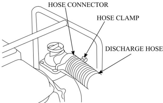
It is best to use a short, large-diameter hose, because that will reduce fluid friction and improve pump's output.
