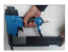
Check that the air supply is at least 60PSI. The gun is now ready to use. Press the head of the gun onto the workpiece to be fastened then squeeze the trigger to fire the nail or staple.
