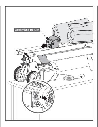
Trigger type lock-out device is adopted to avoid accidental Hydraulic Control Lever pushdown. To operate the Hydraulic Control Lever, draw the Trigger backward with the index finger before pushing the Hydraulic Control Lever forward.
