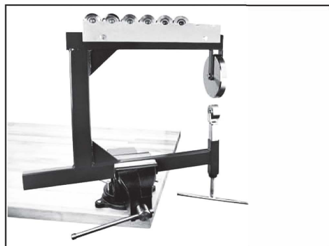
Figure 3. Example of Model 61088 secured in vise mounted to a workbench.
