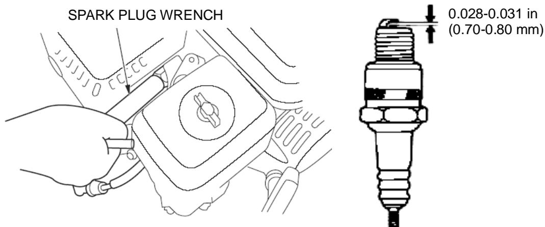
3. Inspect the spark plug. Replace it if the electrodes are worn, or if the insulator is cracked or chipped.
