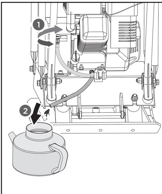
Running the engine with dirty oil can cause premature engine wear and failure. Changing oil regularly is extremely important. The flexible oil drain hose is equipped to drain oil into appropriate receptacle.
