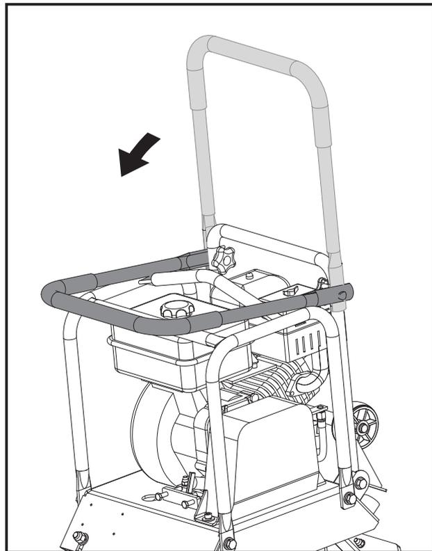
6. Carefully fold the handle down. Do not allow control cables to become pinched or bent.
