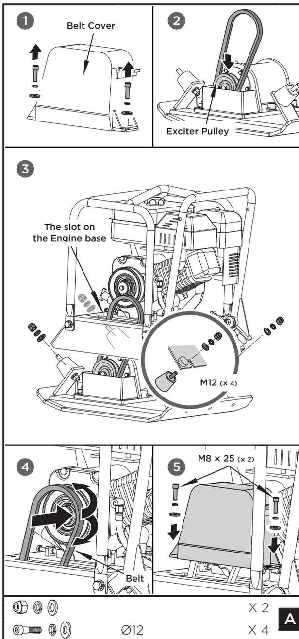
1. Remove the two M8x25 Socket head cap screw from the installed belt cover, set the screws with washers and the belt cover aside for later.
