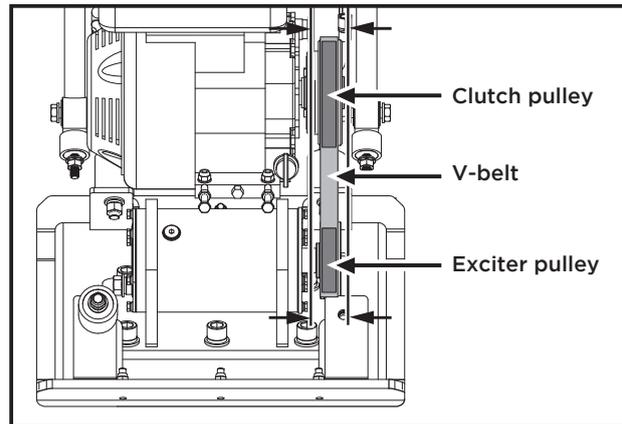
3. Slide the engine toward the front of plate and slip the old V-belt(s) off of the wheel pulley and install the new V-belt(s) in their place.
