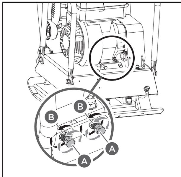
2. Loosen the jam nuts B, leaving enough space between the nut and bracket.
