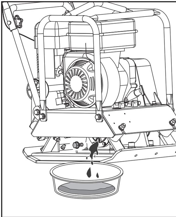
2. Remove bolt plug from side of exciter housing. Tilt the machine side down so oil drains from exciter. Examine oil for metal chips as a precaution to future problems.
