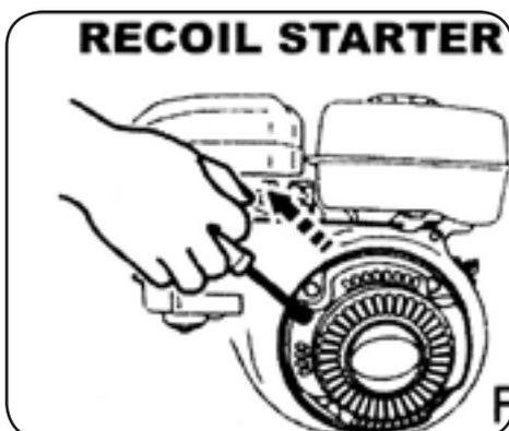
6. **DO NOT** pull out the rope all the way. After starting the engine, allow the starter handle to return to its original position while still holding the handle.
