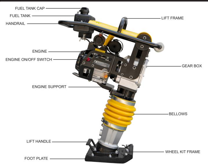
Compact the areas that you would like to work on with the STKUSA Compact Jumping Jack. This machine allows you to condense the that you would be working on to help give the a and compact area for the material to sit atop. Create a ground in your home, yard, or street to help you place
