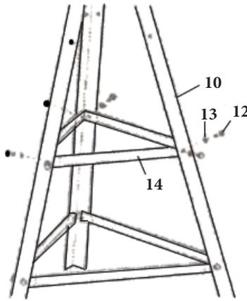
2. Tripod Assembly : Attach the pull rod (11) with the support pillar (10), using the plain washer M8 (13) and bolt M8x16 (12). Attach the short pull rod (14) with the support pillar (10) using the plain washer M8 (13) and bolt M8x16 (12).
