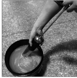
1. Insert the oil reservoir casing into the oil drum and pull the rod to absorb the oil.
