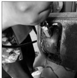
7. Remove the nozzle: Tubing bend to  $35^{\circ}$ , rotate slowly to pull out.
